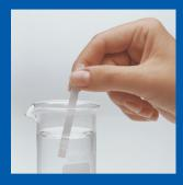
2. The reaction zones are wetted with the solution to be tested simply by dipping them briefly into the liquid sample. Any excess liquid is then shaken off or removed by drawing the test strip across the edge of the vessel.
