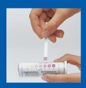
After the specified reaction time of at most one minute has expired, the color of the reaction zone is compared with the color scale printed on the tube label and the corresponding concentration is read.
