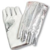
234-AKV-KV Combo glove. 19 oz. aluminized Kevlar®-aramid blend on back for near 2000°F radiant protection. 22 oz. Kevlar®-aramid blend palm for working temperature of 400°F-600°F and good abrasion resistance.
