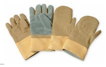
234-AKV-ZP Combo glove. 19 oz. aluminized Kevlar®-aramid fiber blend on back for up to 2000°F radiant protection. 35 oz. Zetex Plus® palm for short duration up to 1800°F. Moderate to poor abrasion resistance.
