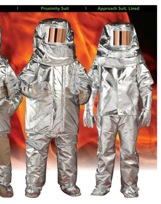
The non-insulated APPROACH suit is used in just about every industry requiring heat protective clothing. It is suitable where ambient temperatures do not exceed 200°F (93°C).
