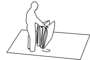
1. Sweep and clear the area where the units will be set-up, cut and lay a protective layer of poly on the floor.
