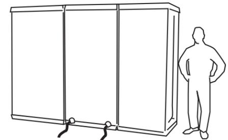
6. For D-Con 2, skip to step 9. For D-Con 3, repeat assembly instructions for the shower unit, note the sump (with blue ports) has an elevated plastic and foam platform to keep the worker out of the drain water. Position the system with shower so that the blue supply and drain ports face the adjacent water source and pump.
