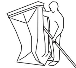
3. Unfold the equipment room unit and stand the unit vertically by lifting the top panel through the entry. Enter the unit and insert the pole set. Pole sets are not included, and are available separately.
