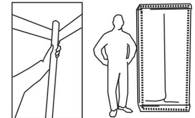
4. Position and tension the poles into the corners, set the poles back from the corner approximately 2-3 inches.
